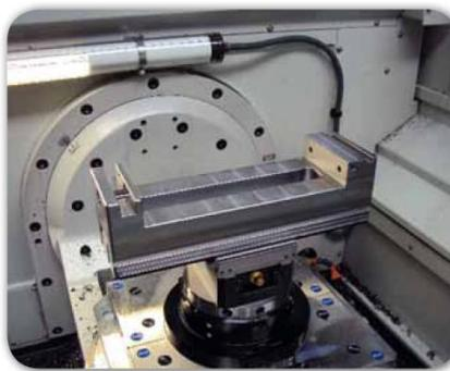
Even long extended parts are held with a clamping depth of only 3 mm.
