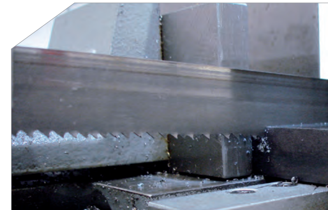
1 Sawing of blank with minimum addition of clamping depth.
