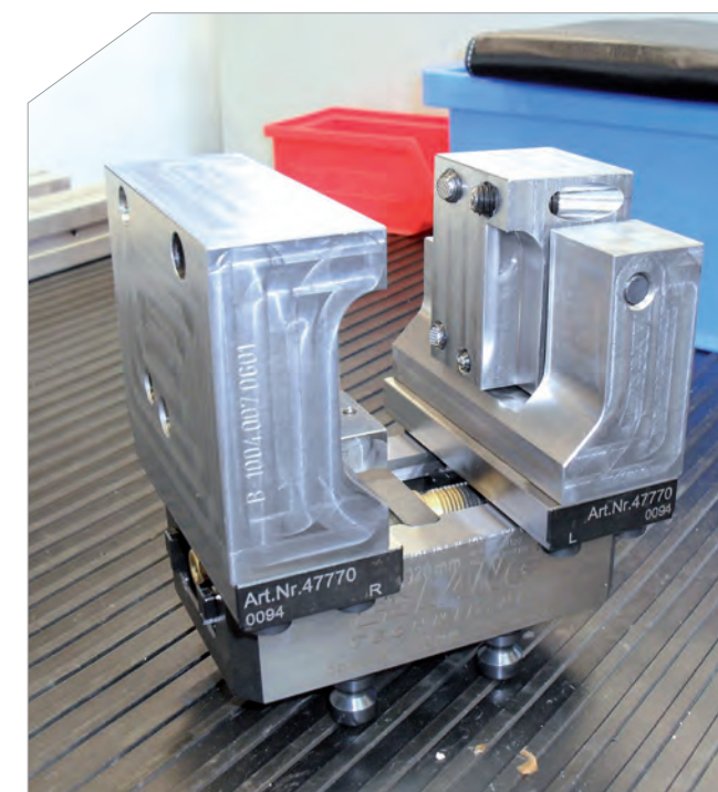
Besides the standard add-on jaws custom-made jaws or fixtures can be mounted on the base jaws! Drawing available upon request.
