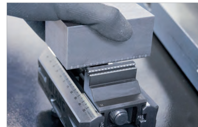
3 Correct stamping depth is reached when the control marks between the holding teeth have a max. depth of 0.1 mm.
