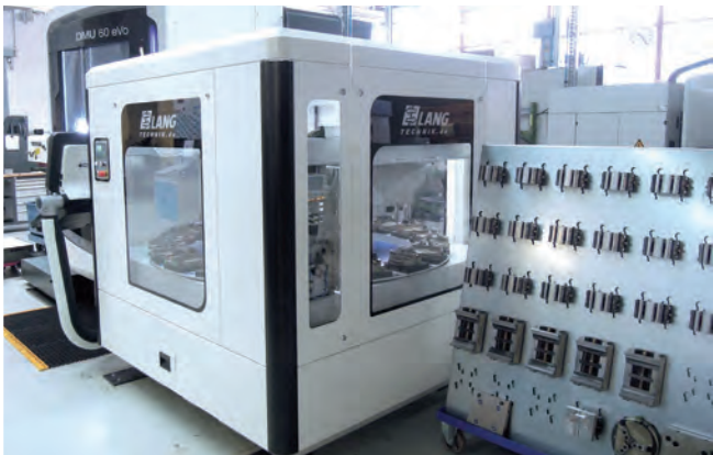
The storage unit can not only hold automation vices but also regular 5-Axis Vices.
