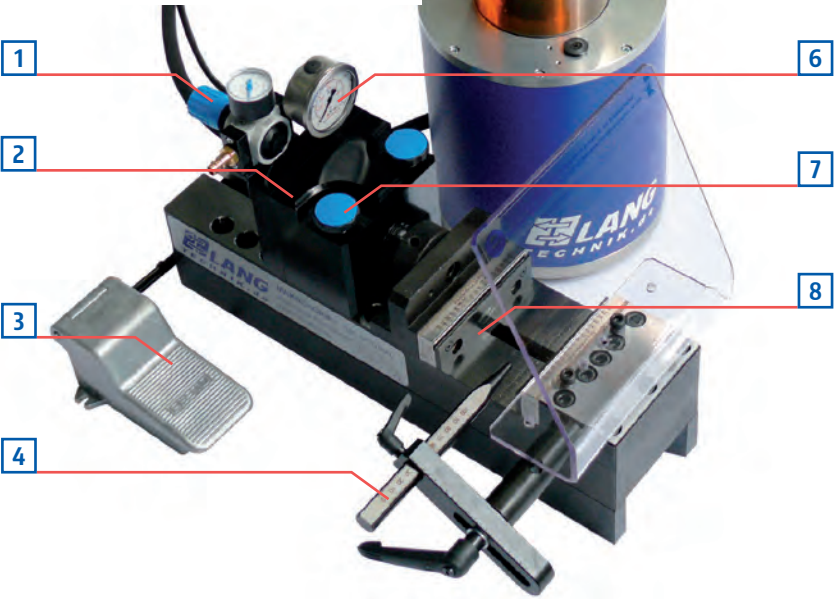
The centre marking tool enables an exact and centric positioning of blanks in 5-Axis Vices - even without endstops. See on page 76.
