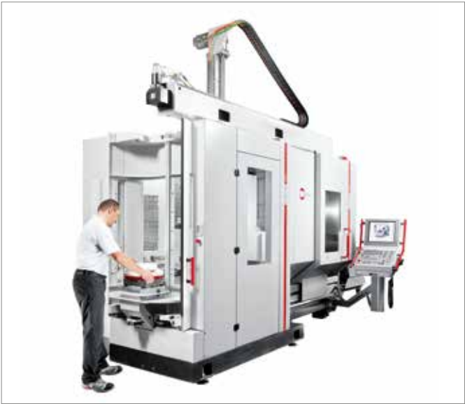
Pallet changer setup station
