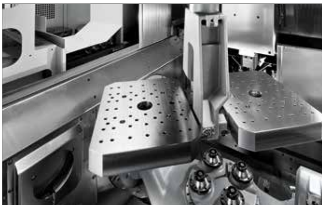
Double gripper for 2 x 100 kg
