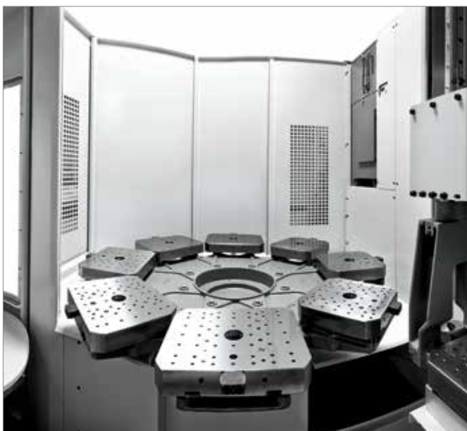
Pallet changer PW 100 with setup station and 8x pallet storage
