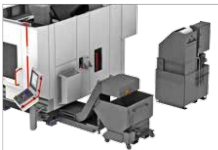
Chip conveyor with internal cooling lubricant supply, right
