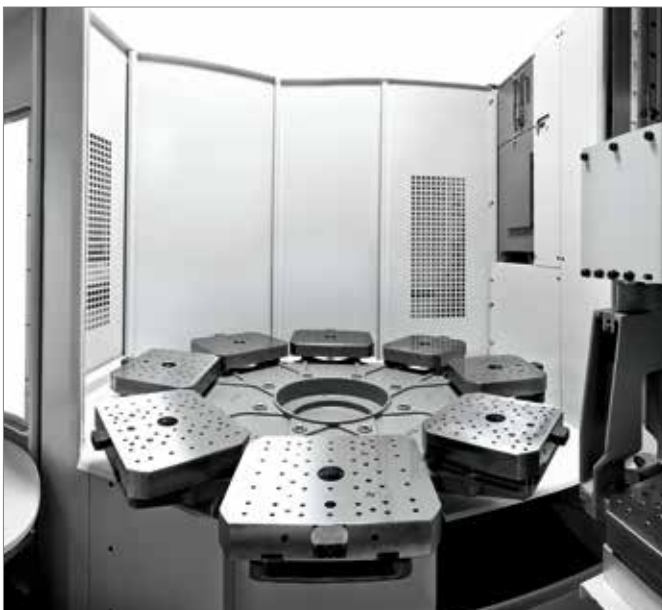
Pallet changer PW 150 with setup station and 8x pallet storage
