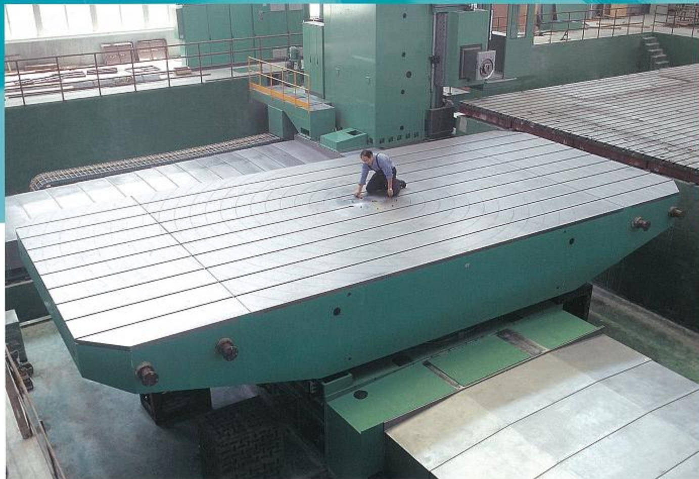
Technical features of hydrostatic rototraversing tables
